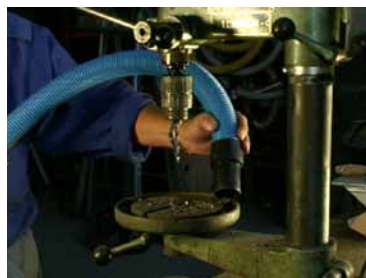
Cleaning of production equipment such as drilling machines, lathes, millers, saws, moulding machines, grinders, etc. It is easy to remove the waste directly at the source – eventually as it occurs.
