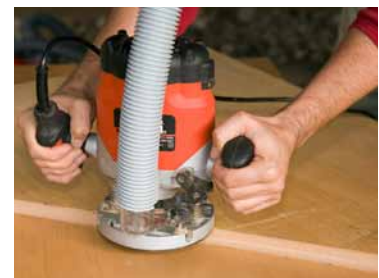
Also in connection with hand tools and the small jobs, it is easy and fast to establish an extraction which effectively removes dust and chips. When it easy – it will get done.
